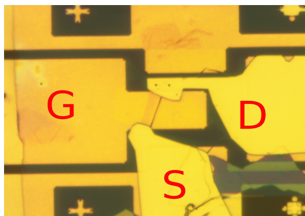
Figure 2 : Detail of a bilayer graphene on hexagonal Boron Nitride transistor on top of a low luminescent quartz substrate. The graphene has a ribbon shape and is sandwiched between the source (S) and the drain (D) electrodes.
