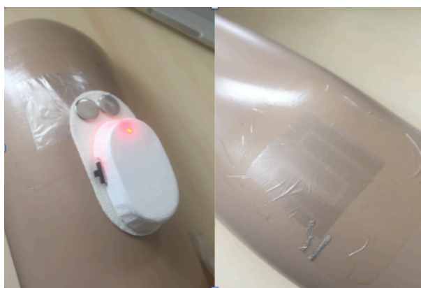
Figure 2 : Graphene on polymer wound dressing with electrical function.
